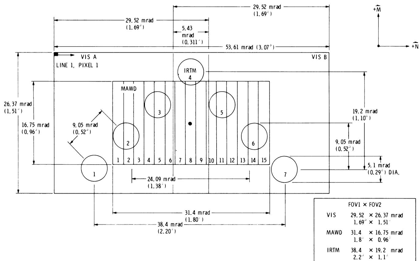
Fig. 6. Fields of view of orbiter instruments.
