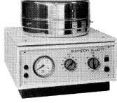
synovial fluid, peritoneal exudates, seminal or other body fluids. Centrifugation and slide preparation are performed simultaneously, which eliminates prior centrifugation and saves you time. Improved head design ensures safety when working with pathogenic organisms.
