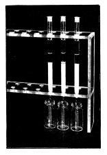
Inexpensive (less than \$2.50 each, evenreuseable) columns of borosilicate glass, prefilled with Sephadex® LH-20, for steroid purifications. System includes special column-holding rack. Handles 20 sample columns at once.
