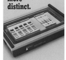
Thin Layer Isoelectric Focusing (TLIEF) is a new separation technique offering numerous advantages over conventional isoelectric focusing. These include simultaneous separation of multiple samples with outstanding resolution, accurate and simple pH determinations, and distinct evaluation by paper print technique.
