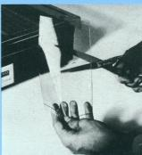
The Ampholine® PAGplate can be used complete for 24 samples, or cut in half for 12 samples and in thirds for 8 or 16 samples. The remaining parts can then be stored in the original package in a refrigerator until your next experiment.
