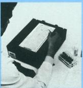
Applying your sample is simple and precise with the sample application pieces. Dip, soak for a few seconds in your sample solution, and then place on the gel surface.
