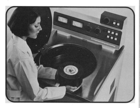
The Sorvall<sup>®</sup> RC-5 refrigerated superspeed centrifuge with a Rate Controller is ideal for density gradient work. The soft start and soft stop characteristics of the Rate Controller prevent mixing of the gradient at speeds between 0 and 1,000 rpm.
