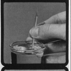
You've probably heard of the technique for filling microelectrodes by inserting a small fiber into the tube before pulling the micropipette. The fiber promotes capillary action facilitating filling.
