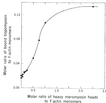
Fig. 2. Induction of binding between tropomyosin and F-actin by HMM at very low salt. Conditions: 30 mM KCl, 1 mM EDTA, 0.045 mg of tropomyosin per milliliter, 0.2 mg of F-actin per milliliter, 1 mM imidazole buffer, pH 7.0, and increasing concentrations of HMM.
