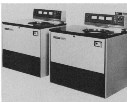
Fig. 1. The OTD ultracentrifuge system has an oil turbine drive that eliminates drag from gears, belts, and reduces uneven bearing loads, vibration, friction, and wear. Other features include temperature control to within 1° from 0° to 40°C.
