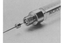
There's a Teflon seal in the hub that can be finger tightened to compensate for wear and to prevent leakage. You simply tighten the knurled hub to make the adjustment for a leak-tight seal. Tested for accuracy Every 7000 Series syringe is tested for accuracy by injecting a series of samples into a gas chromatograph. When you purchase a Hamilton 7000 syringe, yoù have our guarantee that it will deliver the capacity with reproducibility to  $\pm 1\%$ .
