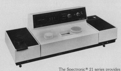
continuous wavelength ranges of 200-1000nm, a narrow 10nm spectral slit width, choice of meter and digital readouts,
