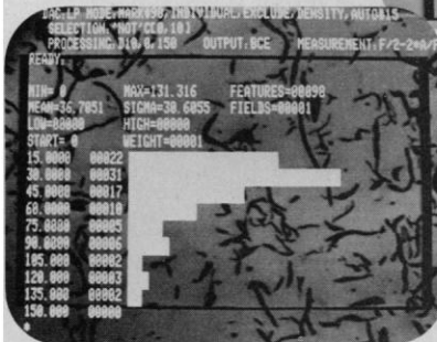
Size distribution of elongated inclusions in a steel sample in accordance with their curved lengths.
