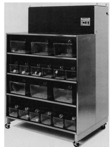
Laminar air flow is a technique which significantly reduces concentrations of airborne contamination in your animal breeding or research area.
