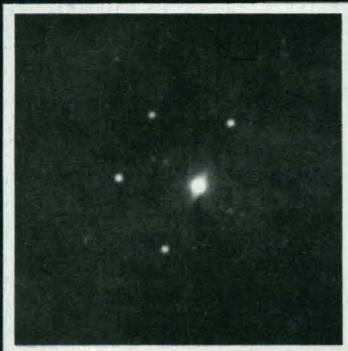
3 SAD using rocking beam mode. Effective aperture less than  $50 \text{ \AA}$ .
