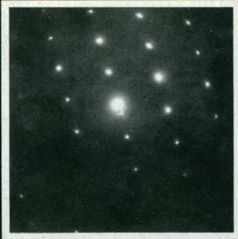
2 SAD by using STEM optics to produce an effective aperture of approximately  $.5 \mu\text{m}$ .
