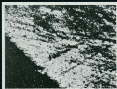
Dark field image of stressed polyethylene using annular detector. 100kV.
