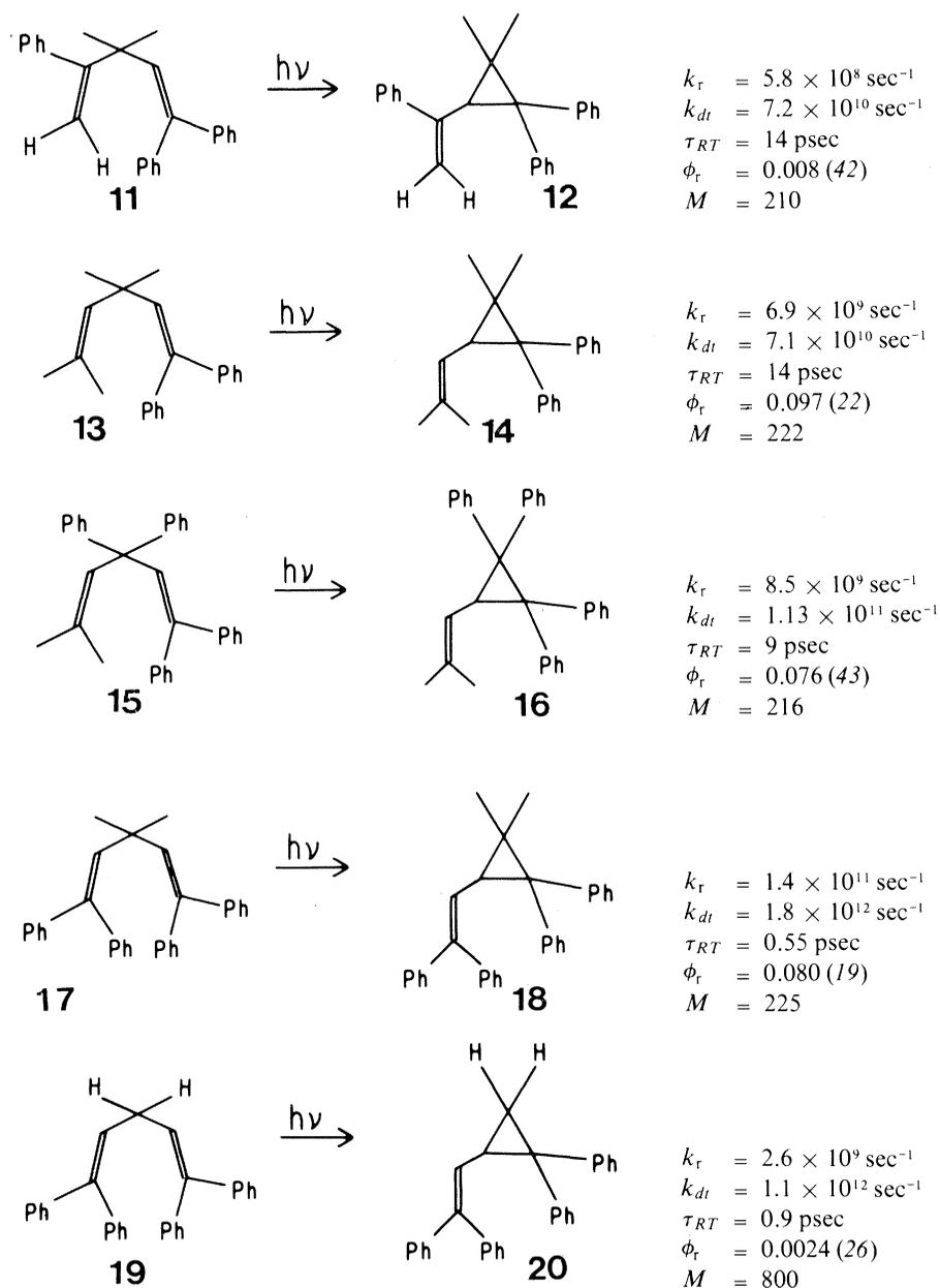
Fig. 2. Some rearrangement rates obtained by single photon counting (30).
