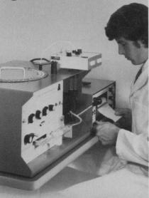
ISCO density gradient fractionators produce a continuous absorbance profile as the gradient is fractionated into a built-in collector. Zones undetectable by other methods are easily resolved and their exact locations plotted. Any size centrifuge tube can be guantitatively scanned at two wavelengths and fractionated with or without piercing.
