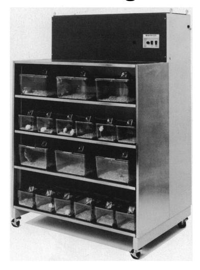
Laminar air flow is a technique which significantly reduces concentrations of airborne contamination in your animal breeding or research area.
