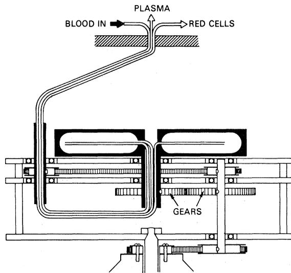
boscopic illumination. Three silicone rubber tubes from the rubber bag are led down through the center of the centrifuge bowl, then upward through the hollow shaft, and finally through the center hole of the centrifuge cover where they are tightly supported. When properly balanced, the centrifuge bowl can be operated at speeds up to 2000 rev/min.
