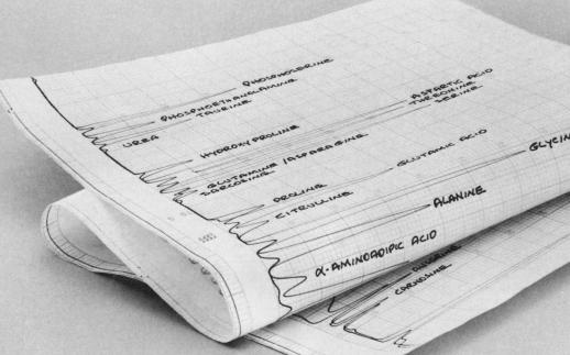
Now you can analyze physiological fluids in only 4½ hours on the Model 121M Microcolumn Amino Acid Analyzer. This 2-column method, using sodium citrate buffers, takes less than half the time required by many older methods.
