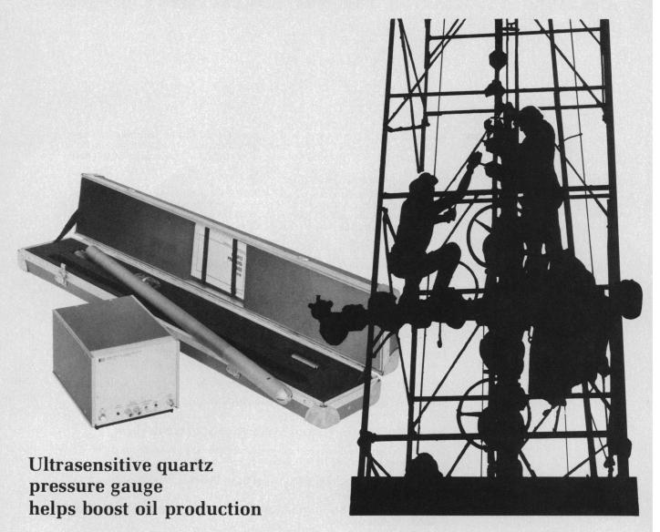
Able to measure a change as small as 0.01 psi at wellbore pressures up to 11,000 psi, the HP 2811B helps engineers evaluate reservoir parameters for optimal oil recovery.
