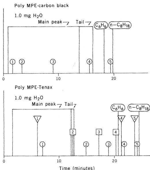
Fig. 1. Plots of retention time illustrating the superior resolution of organic species from water on the Poly MPE-Tenax column. Circled numerals indicate carbon numbers in the homologous series of alcohols, squares represent aldehydes, and triangles represent amines. The Poly MPE-carbon black column does not provide well-defined peaks for amines and aldehydes. Conditions are as specified in Table 1.
