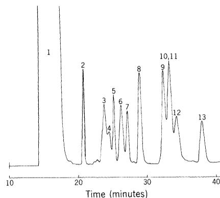
Fig. 2. Chromatogram illustrating the resolution of 12 representative compounds on a Poly MPE-Tenax column. Conditions are as specified in Table 1. Key: 1, isopropanol (solvent); 2, benzene; 3, dimethyl furan; 4, octane; 5, isopentyl alcohol; 6, nonane; 7, furfuryl alcohol; 8, mesitylene; 9, *p*-cresol; 10 and 11, tridecane and dimethylaniline; 12, phenethyl amine; and 13, benzyl cyanide.
