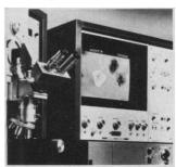
The Quantimet 720, by offering a wide selection of automated image analysis capabilities, enables the scientist to perform sophisticated, reproducible and accurate measurements at speeds up to 1,000 times faster than by conventional methods.
