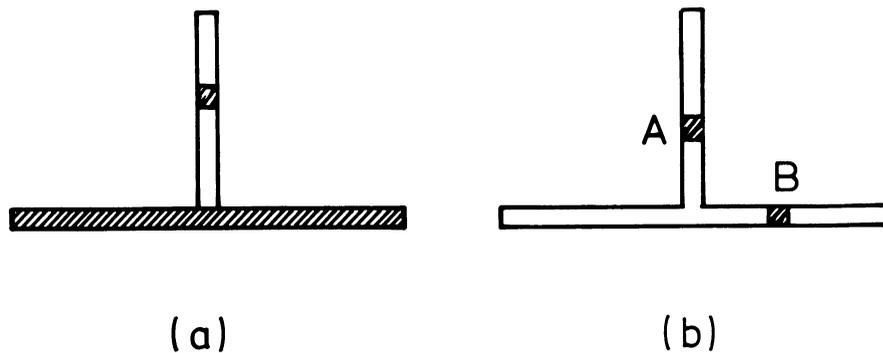
Fig. 2. (a) The arrangement used in the instrument built in 1954 by J. H. Blythe. (b) The equivalent instrument using two small elements.
