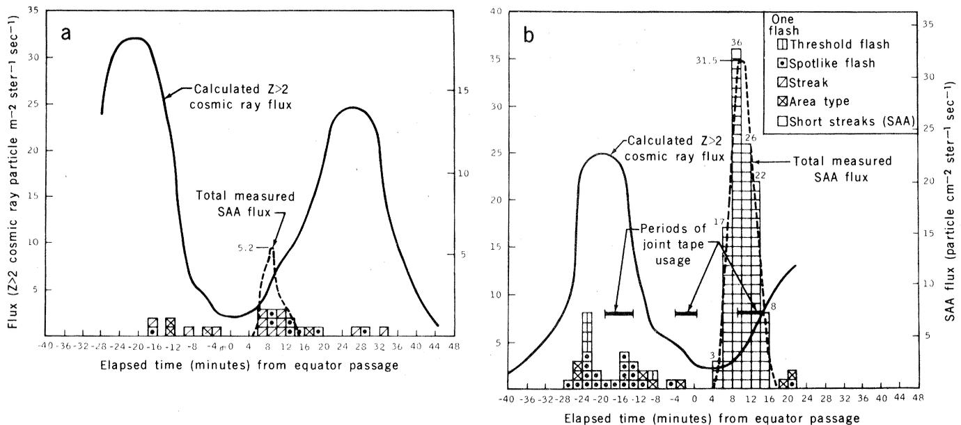
Fig. 1. Results of the first light flash observing session (a) and the second light flash observing session (b). Individual flashes are represented in histogram fashion versus time and compared with the calculated  $Z > 2$  primary cosmic-ray flux (left scale). Also shown (dotted line referring to the right scale) is the measured  $Z \geq 1$  SAA flux for each session. The types of events are indicated schematically.
