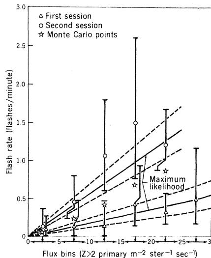
Fig. 2. The flash rate outside the SAA is plotted for each of the flux bins (each 5.0  $Z > 2$  particles per square meter per steradian per second wide) indicated. The total observing time and the number of flashes seen while in each flux region were compiled for each session, and the errors reflect the differing amount of time spent in each flux region. The maximum likelihood errors are indicated by the dotted lines which represent one standard deviation from a two-parameter linear function.
