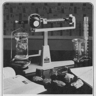
**Dial-O-Gram 310:** direct reading, engraved dial and vernier, magnetic damping, center indicating, windowed poises and only 2 tiered beams provide very high speed, accurate readings. Send for FREE Catalog!
