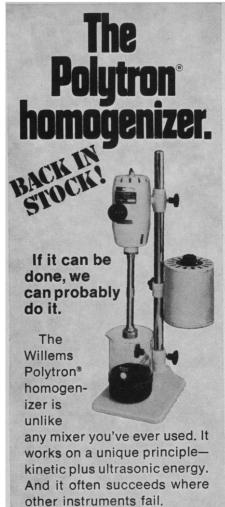
Homogenization by sound waves means that tissues are broken down quickly to subcellular level without destruction of enzyme activity. You'd be hard-pressed to do that with other kinds of mixers.
