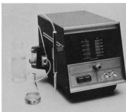
Fig. 1. The ADP-30SD offers precision and reproducibility better than one part per thousand. It is useful in radioimmunoassay protocols.
