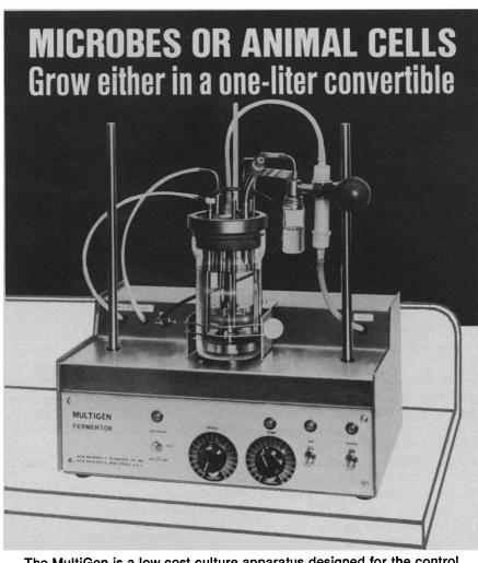
The MultiGen is a low cost culture apparatus designed for the control of all basic environmental conditions: temperature, agitation, aeration, pH, and dissolved  $O_2$ . Whether the need is for viscous microbial cultures or animal cell suspensions, air sparging or gas overlay, the MultiGen can be adapted to specific research requirements, and can provide an ideal alternative to spinner flask procedures.
