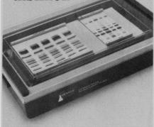
Thin Layer Isoelectric Focusing (TLIEF) is a new separation technique offering numerous advantages over conventional isoelectric focusing. These include simultaneous separation of multiple samples with outstanding resolution, accurate and simple pH determinations, and distinct evaluation by paper print technique.
