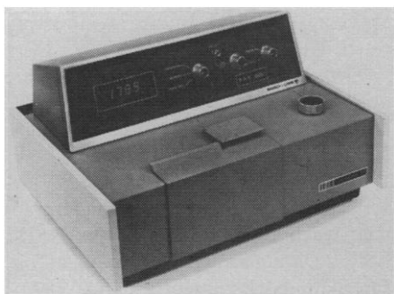
Fig. 1. The Bausch & Lomb Spectronic 710 provides digital readout in three modes and features binary coded decimal output as well.
