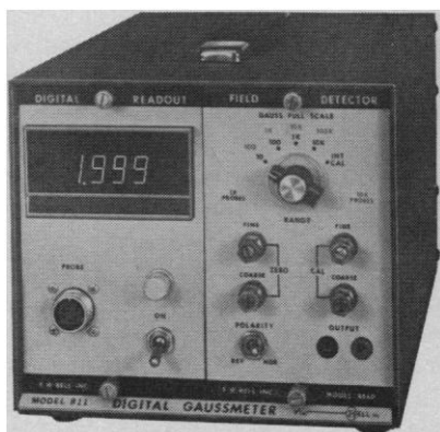
Fig. 2 (left). The 811 digital gaussmeter is available in bench cabinet or rack-mounted configurations. It measures magnetic flux density in five ranges. Fig. 3 (right). Temperature controllers and circulators of the 1400 series from B. Braun Instruments rely on electronic sensors. They offer stability, high heating capacity, and several temperature ranges.
