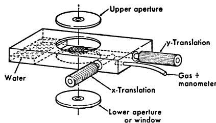
Fig. 6. Slide hydration chamber which permits microculture of cells on an electron microscope grid to be examined in either the light microscope or the electron microscope. The drop of medium on the grid can be changed by removing the upper aperture and the drop thinned down prior to electron microscopy.
