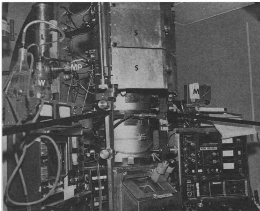
Fig. 5. Differentially pumped environmental chamber fitted to the U.S. Steel 1.0-Mev electron microscope (designed by V. R. Matricardi). Abbreviations: *MP*, mechanical pump connection; *L*, liquid nitrogen trap; *M*, manometer measuring water pressure in the chamber and thermocouple measuring the wet specimen temperature; *W*, humidified air inlet for bringing the chamber up to a pressure of 1 atm before the insertion of a specimen; *S*, x-ray shielding.
