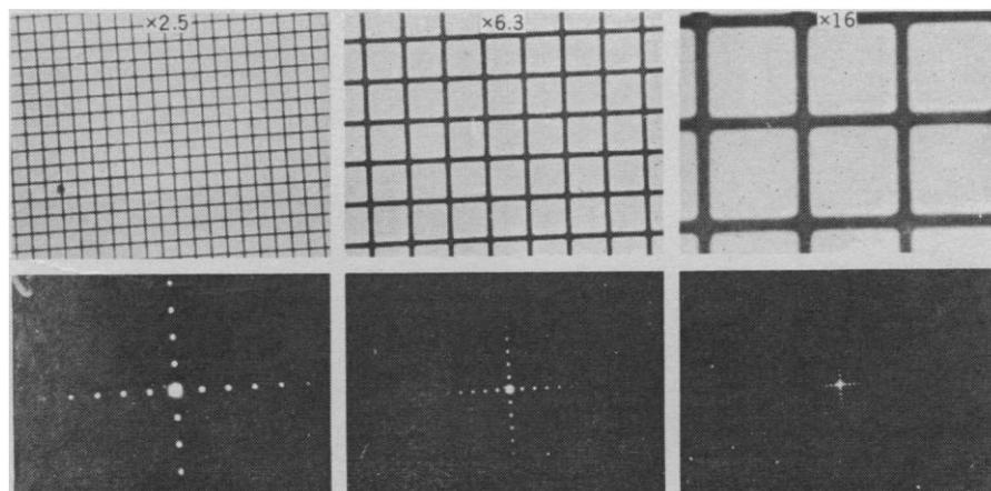
Fig. 5. Photomicrographs (top) and diffraction patterns (bottom) used to calibrate the microscope system for  $\times 2.5$ ,  $\times 6.3$ , and  $\times 16$  objectives. The actual spacing of grid elements is 10 lines per millimeter.
