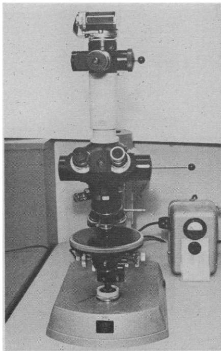
Fig. 4. Microscope arrangement used to generate and photographically record diffraction patterns generated directly by petrographic thin sections. The arrow indicates the position of the filter assembly that yields quasi-monochromatic, partially coherent light from a mercury vapor source.
