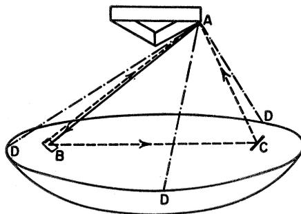
Fig. 4. Schematic of the laser survey method. The laser and its steering mirror are at *A*, the panel target at *B*, the surface steering mirror at *C*, and the reference targets at *D*; hence *CA* is on a radius of the sphere.
