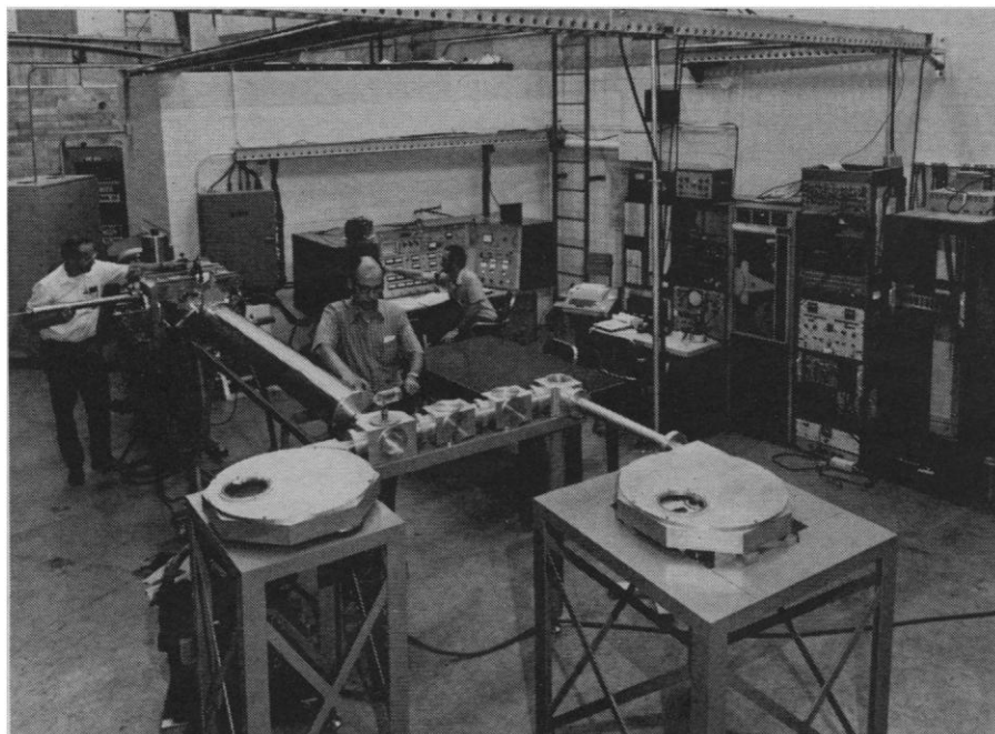
Fig. 1. UNISOR laboratory wing on the Oak Ridge Isochronous Cyclotron (ORIC) building. The target and ion source is behind the wall in the upper center, the separator control console is in the center, and the end of the separator magnet and the collection box are on the left, with the extracted beam tube leading to the tape transport unit in the foreground. There are four detector stations on the tape transport unit. In operation, this area is filled with detectors and shielding. The new Tennecomp system is installed now where the older systems are on the right in the photograph.
