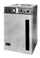
Here is the new generation in incubators — a water-jacketed, automatic  $CO_2$  control incubator with a "closed-loop" control system that provides a stable air/ $CO_2$  environment, reducing  $CO_2$  consumption and giving extremely accurate results from direct-dialed settings. National's new automatic  $CO_2$  control water-jacketed incubators has these fine features:
