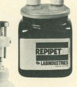
3. NEW REPIPET Jr. Dispenser only \$29.50. An unbreakable plastic 0.5% precision dispenser for non-corrosive reagents. We include chemical resistance chart.
