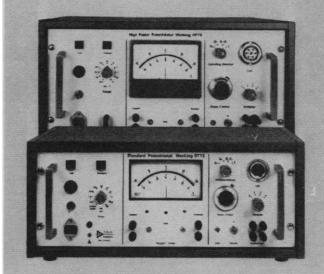
"Versatile" is the only way to describe the new Wenking Potentiostats. Both the new High Power Model (HP-72, 200W output) and Standard Model (ST-72, 75W output) provide the flexibility of higher output voltage (at medium current) or higher output current (at medium voltage) simply by adjusting a multipin connector at the back of the instrument.
