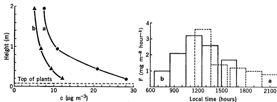
Fig. 1 (left). Profiles of ammonia concentration,  $c$ , over an alfalfa pasture: profile a, 1600–1800 hours on 14 March 1974; profile b, 1500–1700 hours on 15 March 1974. Fig. 2 (right). Flux densities of nitrogen (as ammonia and related compounds),  $F$ , from pasture: profile a, 14 March 1974; profile b, 15 March 1974.
