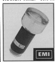
EMI has added a 3" linear focused tube to its range of 3/4" and 2" tubes. The unique 9821 incorporates a computer designed front end to ensure maximum collection efficiency. Fitted with 12 dynodes having BeO secondary emitting surfaces, the 9821 gives a typical gain of 4 x 10<sup>7</sup> at 2800 volts. The high efficiency bialkali cathode also ensures a low dark current level (typically 3 nA at 200 A/Im) required for certain applications.
