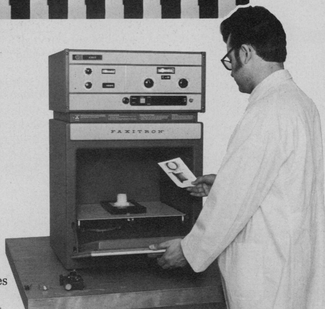
The HP 43805 cabinet X-ray system gives you correctly exposed films automatically—like these radiographs of a defective printed circuit board and an aluminum casting.
