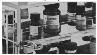
FRIGICATOR replaces the old vacuum desiccator which takes up space and is awkward to use. It's air-tight, light-weight, easy to open, and spacesaving, with slide-out trays for easy organization. Fits handily in refrigerator, freezer, or on a bench. FRIGICATOR (9" x 9" x 16") is constructed of 1/4" transparent acrylic. Shipped F.O.B. Omaha (desiccant included) for \$76.
