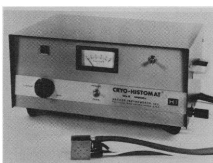
Fig. 3 (top left). Delta Data Systems manufactures this model 5500 video display terminal. It has a 2048-character buffered memory and displays up to 27 lines of 80 characters each. Fig. 4 (top right). The Cryo-Histomat MK-2 from Hacker Instruments provides rapid freezing of tissue samples for microtomy and rapid reversal of polarity to allow specimen removal or repositioning. Fig. 5 (bottom left). International Light offers the IL 500 radiometer for power measurement in the range of 200 to 800 nanometers. Readout is in watts or watts per square centimeter.
