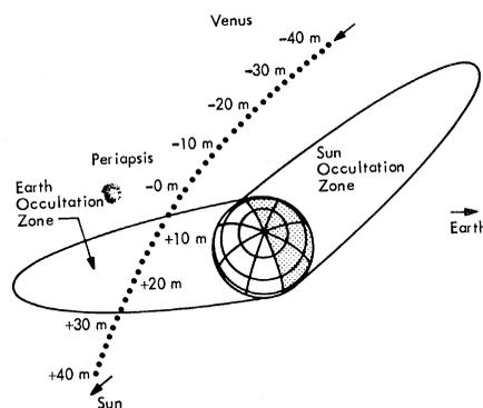
Fig. 2. Venus close flyby geometry, viewed from the trajectory north pole. Dots show spacecraft position at 2-minute intervals. Spacecraft altitude at periapsis was 5785 km.
