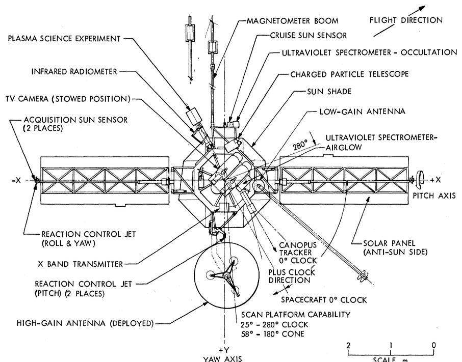
Fig. 1. The Mariner 10 spacecraft looking sunward along the spacecraft Z axis (normal to the plane of the drawing at the intersection of the X and Y axes). The dashed line drawing of the low-gain antenna shows its position for the extended mission, which starts approximately 2 weeks after Mercury encounter.
