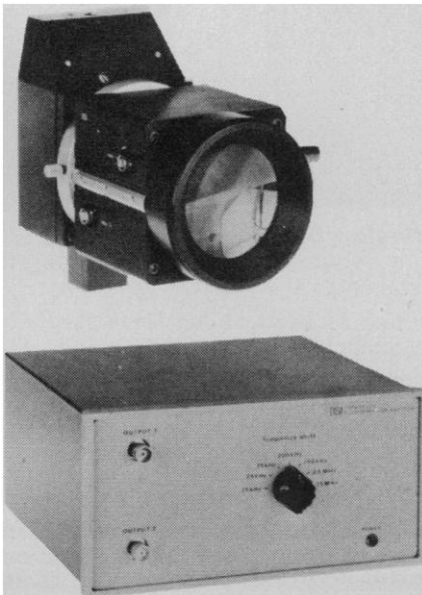
Fig. 1 (above). The Cahn model 4600 electro-balance offers portability and the capacity for remote control operation. It will accommodate a maximum load of 2.5 grams. Its sensitivity is 0.0001 milligram. Fig. 2 (right). Flow direction adaptor kit for the Laser Doppler Anemometer from Disa Electronics extends the anemometer's versatility.
