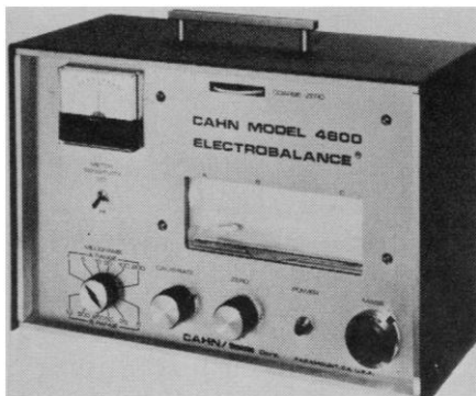
Fig. 1 (above). The Cahn model 4600 electro-balance offers portability and the capacity for remote control operation. It will accommodate a maximum load of 2.5 grams. Its sensitivity is 0.0001 milligram. Fig. 2 (right). Flow direction adaptor kit for the Laser Doppler Anemometer from Disa Electronics extends the anemometer's versatility.
