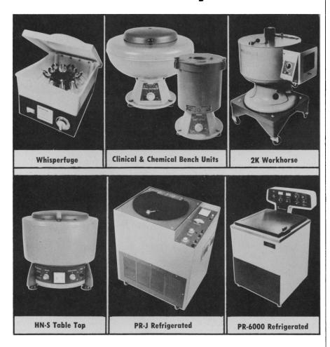
Seven of the fifteen different IEC centrifuges we stock are pictured here. Models range from the "Whisperfuge" - a table-top centrifuge costing only \$195.00 with a rated capacity of 180 ml (12x15) that operates at two speeds (3000 rpm/1000xg and 2000 rpm/500xg) and is capable of performing twenty-four tests with three complete washes in seven minutes . . . to the PR-6000 priced at \$3,360.00 which provides blood banking, generalpurpose, and even some ultra-centrifuge capabilities.
