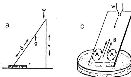
Fig. 1. (a) Diagram of experimental apparatus; *r*, reservoir with water and spores; *g*, glass strip; *w*, point of water application; *d*, distance from source traveled by spores; *v*, vertical distance traveled by spores. (b) Diagram showing surface motion of spores on water; *A*, rapid circulating motion; *B*, slow or rapid movement of spores toward water source at *w*.
