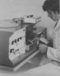
ISCO density gradient fractionators produce a continuous absorbance profile as the gradient is fractionated into a built-in collector. Zones undetectable by other methods are easily resolved and their exact locations plotted. Any size centrifuge tube can be quantitatively scanned at two wavelengths and fractionated with or without piercing.
