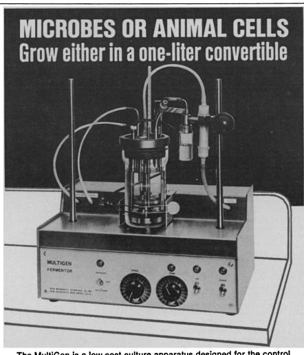
The MultiGen is a low cost culture apparatus designed for the control of all basic environmental conditions: temperature, agitation, aeration, pH, and dissolved O₂. Whether the need is for viscous microbial cultures or animal cell suspensions, air sparging or gas overlay, the MultiGen can be adapted to specific research requirements, and can provide an ideal alternative to spinner flask procedures.
