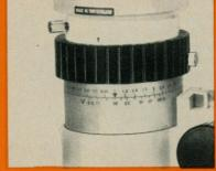
Zoom power changer scale "V" and rotating scale with exposure factors: Once an exposure time has been found for a given power (by trial and error), the accurate exposure time for any other power is simply read off the scale, as long as object and illumination remain unchanged.
