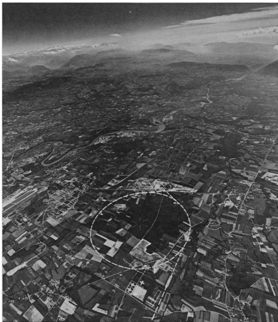
Fig. 1. Aerial view of the Rhone valley near Geneva, Switzerland, looking south into France. The heavily developed triangle of land in the center of the photo is the site of Laboratory I at CERN, including the 28-Gev proton synchrotron, the intersecting storage rings, and associated experimental areas. The dashed lines indicate the location of the new 400-Gev accelerator now under construction. Protons will be initially accelerated to 10 Gev in the small synchrotron, injected into the larger machine where they will move in a clockwise direction around the ring, and then directed either toward the west experimental area (at the tip of the triangle in Laboratory I) or toward the north experimental area at the bottom of the picture. The location of the buildings that will house Laboratory II are also indicated near the north experimental area. The French-Swiss border runs diagonally across the main ring of the accelerator. The international character of the site is further emphasized by the arrangements for utilities: cooling water for the facility will be piped from Lake Lemman in Switzerland, and electric power will come from the French power grid. [Source: European Organization for Nuclear Research]
