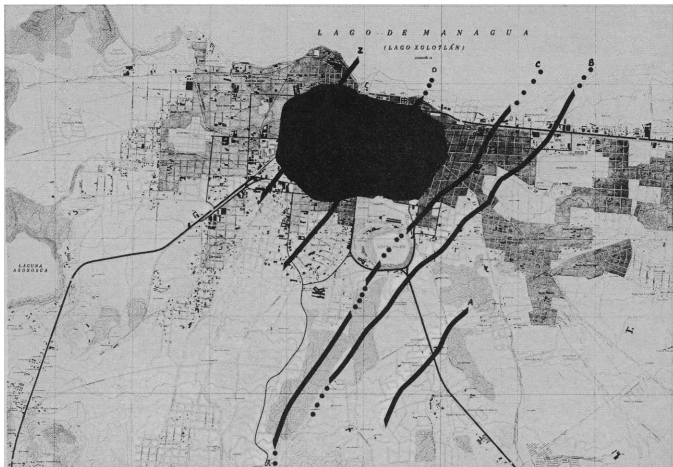
Fig. 3. The shaded area is the estimated area of greatest damage. Lines A-D indicate major faults from December 1972 earthquake. Line Z indicates the major fault from the March 1931 earthquake. A solid line is a fault trace identified in the field, a dotted line is inferred only. [Based on preliminary data from U.S. Geological Survey]
