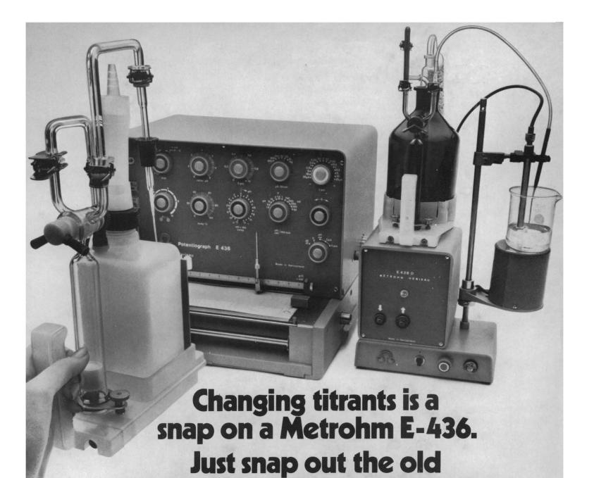
The Metrohm isn't only the world's finest recording titrator. It is also the only automatic titrator with interchangeable, snap-in buret units, and nine buret sizes; from 0.2 ml. to 50 ml. On the E-436 you can do non-stop titrations and change titrant as often as you like. There's no need to constantly stop, disassemble and clean burets, as on instruments with dual systems. Simply replace one buret unit with another and keep right on going.
