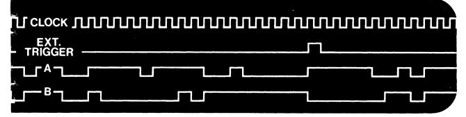
pare it against truth tables or system timing diagrams, you have to learn how the procession of logic states changes with each pulse of the circuit clock.
