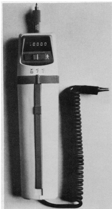
Fig. 1. Model 970A digital multimeter weighs 7 ounces and measures resistance and voltage in a-c or d-c circuits.
