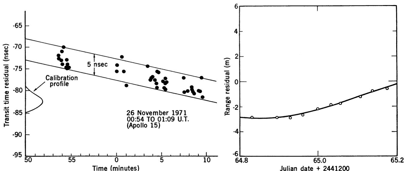
Fig. 5 (left). Individual range residuals (observed minus calculated) obtained over a 20-minute period. The scatter is consistent with that expected from the laser pulse length and the photomultiplier jitter. Fig. 6 (right). Average range residuals obtained during a series of runs covering an interval of 10 hours. The "short-arc" theoretical curve fit to the data gives 11-cm root-mean-square residuals. The time scale is in Julian days.
