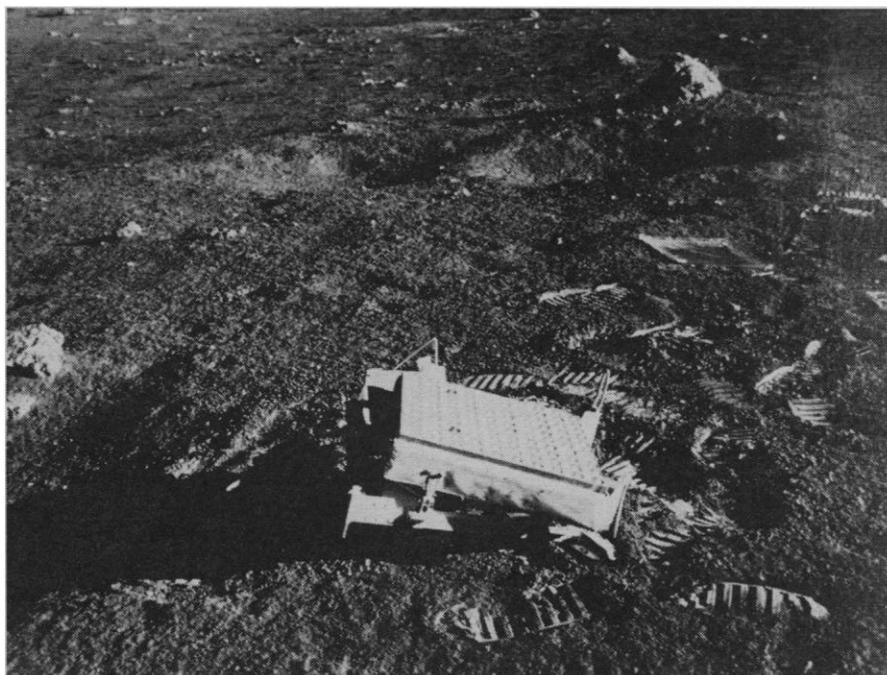
Fig. 3. Apollo 14 reflector package after installation at the Fra Mauro landing site.
